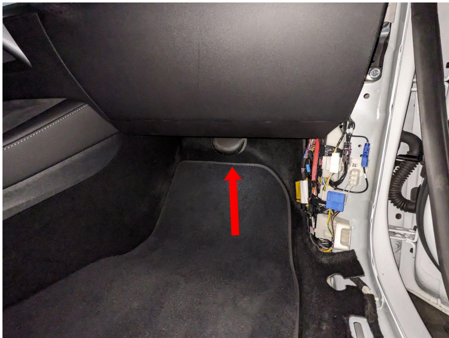
The next step is to remove the panel in the footwell
