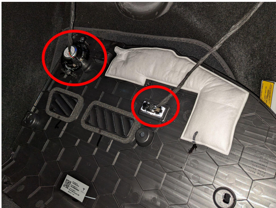
The cables should be unplugged so that the panel can be placed to one side.
